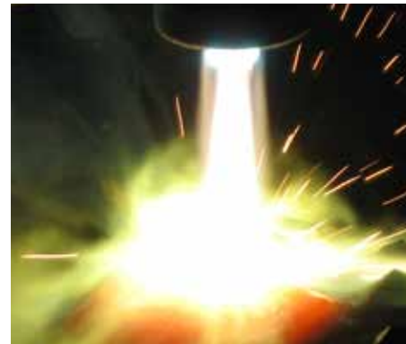
(image) Colferoloy 139 being applied to a wear plate
